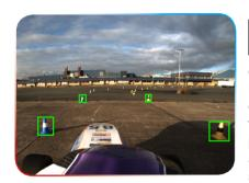
Good machine perception is highly dependent on data acquisition by "exteroceptive" sensors; these are sensors that perceive a machine's environment. The Driverless Formula Student competition has tracks laid out with blue and yellow traffic cones on either end. These cones provide the only reliable source for navigation for the race car. In order to sense both the position and color of the cones robustly, we use a combination of a camera and so called "LiDAR"
